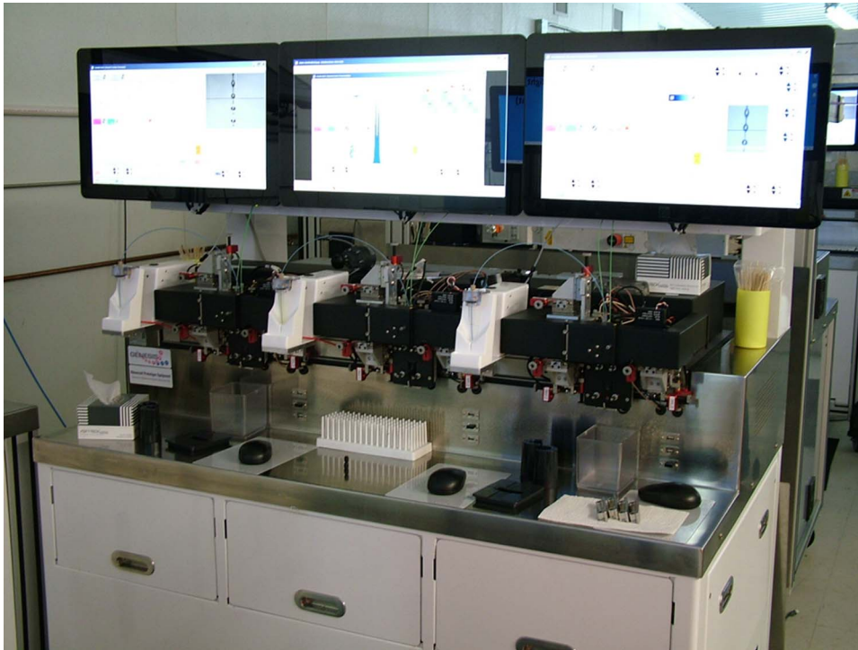
Figure 6 The new Genesis III a modular high-speed sorting platform for parallel processing. Banks of five Genesis III machines are set up in a pod for fast throughput. The speed of sorting in a pod can reach up to 500 million cells/h.
