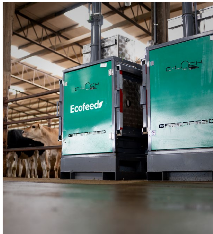
Breathe analyzers are used to measure methane, oxygen, and carbon dioxide emissions of individual animals.
